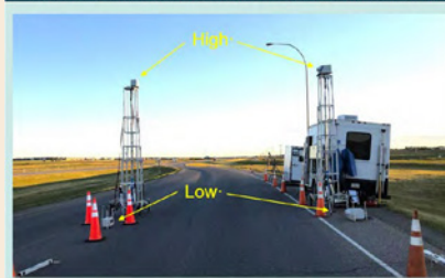
Figure 4: Two attended RSD3000s deployed at different heights to measure HDVs
